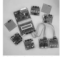
supply), a CPU with serial RS-232 interface and a 16x2 LC-display (optional). 'eLABbase' consists of the all programmable 'dlk51' development platform, the eLAB2dlk51-adapter attached to it (with optional LC-display) and a housing (optional). The size of the module with housing is 178x114x32mm (LxWxH). Programming of active eLAB modules is done via 'eLABbase'.
